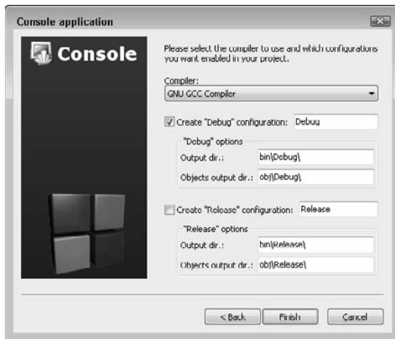
Figure 20-1: The Console Application dialog box of the Project Wizard allows you to select whether to build a debug version of the executable or not.
