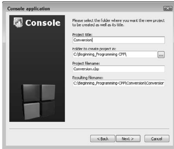
Figure 3-1: The Project window for the Conversion program.
